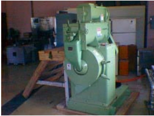
Figure 1. Compression pellet mill used to make experimental tilapia diets.
