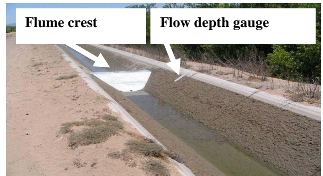
Improved accuracy in water measurement and control allows accurate quantification of irrigation efficiency and deep percolation losses
