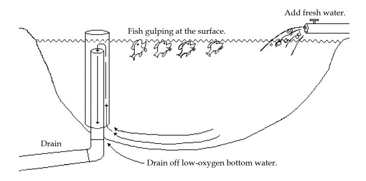
Figure 6: A fish pond with low oxygen.
