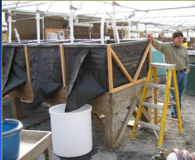
The normal operating procedure for geotextile bags is to pump them full with sludge and allow the sludge to slowly dewater and drain out of the porous bag. This works well with sludge that has a high solids content (10 to 30% solids), but initial tests showed that for the solids content of aquacultural wastes (0.1 to 1% solids) insufficient solids were deposited in the bags during each fill/drain cycle.
