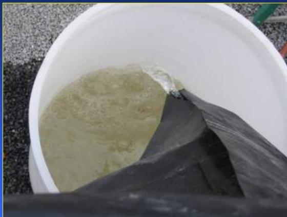
Test procedures were similar to the hanging bag tests with the addition of a paddlewheel flow meter and totalizer that allowed accurate dosing of each bag. For each test, approximately 75 L of wastewater was pumped into three bags at 18 Lpm flow rate. The bags were then allowed to settle and the process repeated
