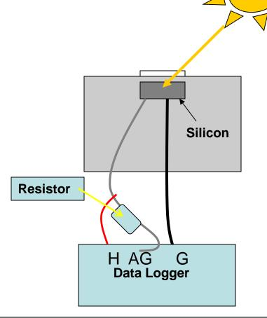
Silicon cell converts solar energy into an electrical current. The current is forced across a resistor to generate a voltage drop which is measured by the data logger.
