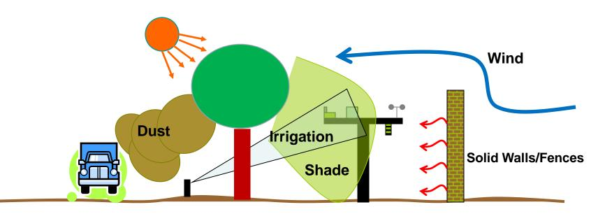
Adjacent roads/parking lots generate dust, heat & potential for vandalism. Shade reduces level of soil radiation measured. Solid walls & fences reduce wind speed and generate heat. Irrigation produces higher humidity, cooler temperatures and false rain events.
