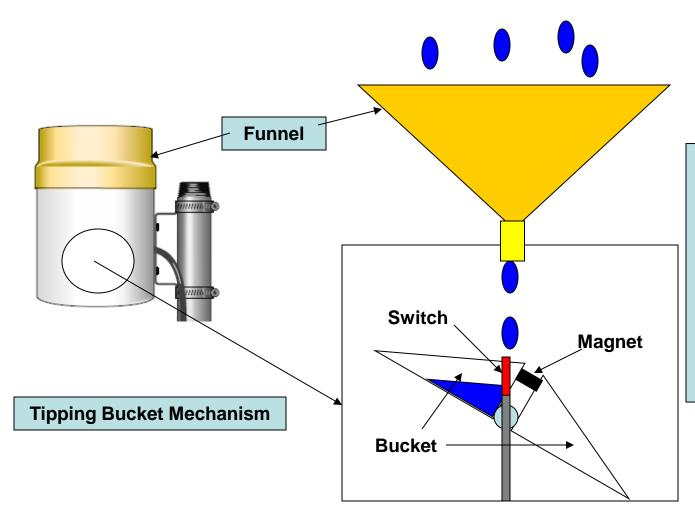
Funnel directs rainfall into tipping bucket mechanism. When one bucket accumulates 0.01" of water, the mechanism tips which causes the magnet to trip a small switch. This switch closure is counted by the data logger as 0.01" of precipitation.
