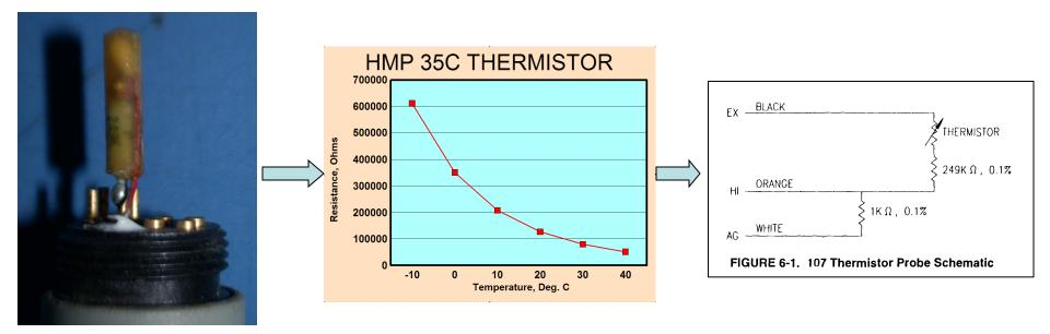
Thermistors are temperature sensitive electrical resistors. They are typically placed in a simple half bridge electrical circuit. As the temperature changes, the voltage drop across the thermistor changes and is measured by a data logger or voltmeter.
