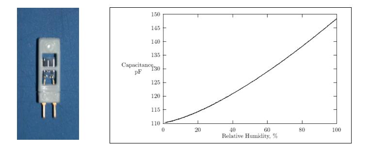
Electrical Capacitance of Sensor Changes With Humidity. When Sensor Is Installed In Proper Electrical Circuit, Voltage Output of Sensor Changes Linearly With Humidity. The Voltage Is Measured With The Data Logger
