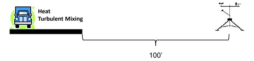
Heat from concrete/asphalt can be advected downwind to station. Passing vehicles create turbulence and create effects similar to wind machines
