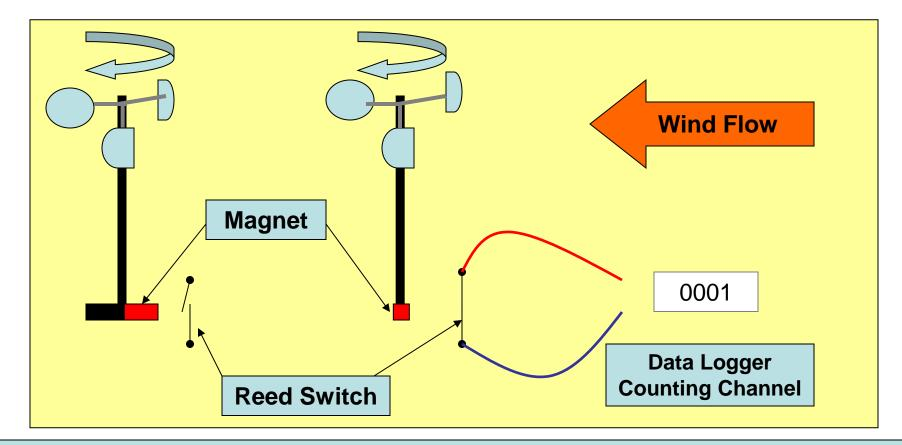
Wind rotates cups and attached magnet which is located adjacent to a reed switch. The rotating magnet opens and closes the switch. The data logger counts the number of switch closures over a defined period of time.
