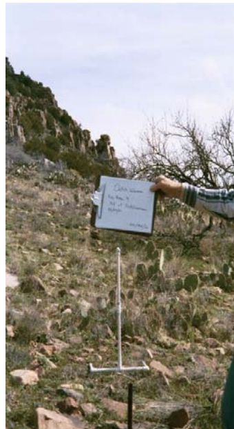
Figure 6. Just below the clipboard is located a stake from an old Parker-3-Step transect. Since some historical data is available, a key area was located at the location of the old Parker-3-Step. This cluster was located at the high elevation part of the ranch. Several hours were expended to try and locate this old cluster. When the key area is read in succeeding years, it will be a good idea to pinpoint this key area with GPS coordinates.
