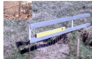
Figure 2. Soil Erosion Bridge (SEB). Two horizontal bars are placed between fixed vertical steel rods. Pins are then used to measure microtopography and surface changes (inserted image).
