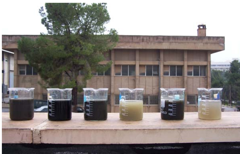
Figure 4: Appearance of septage collected from tankers discharging to the decentralized septage treatment plant at Tal Al Mantah (January 2005).
