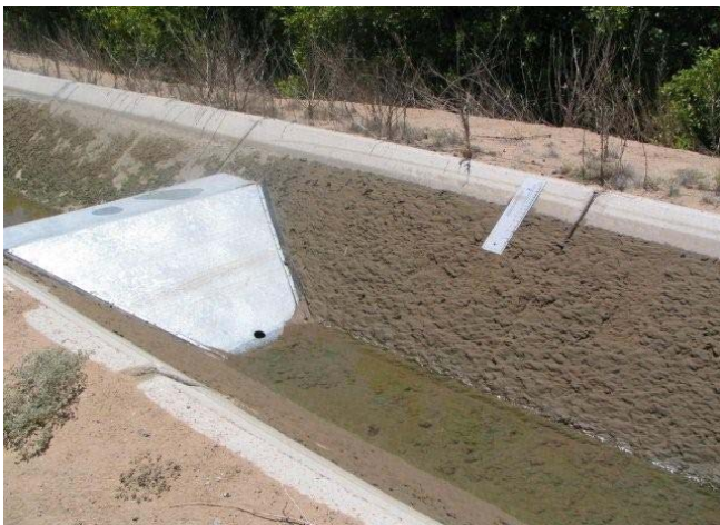
Water measuring flume installed in the field water supply channel of a grower's farm to help raise irrigation application efficiency
