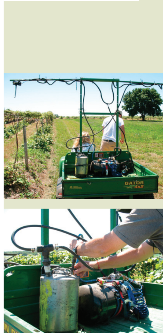
Fig. 4. Gator-mounted mechanical applicator for treatment of vineyards with SPLAT-GBM. Width of the applicator boom can be adjusted for different trellis systems and row spacing (top). Close-up of refillable air tank and SPLAT canister (bottom).
