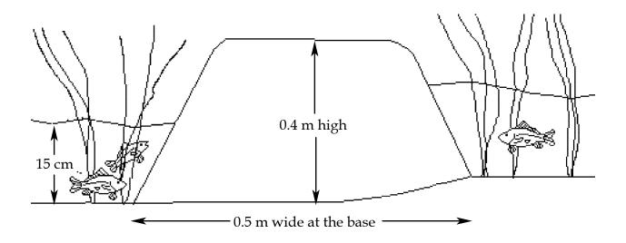
Figure 3: Dike measurements.
