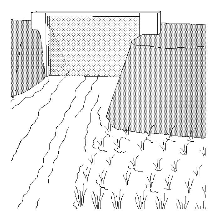
Figure 4: Screens are placed across paddy inlet and outlet areas.
