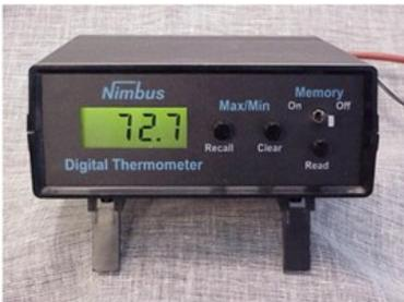
inside the house and is continually updated to display the current temperature. It also remembers the highest and lowest temperatures since it was last reset. Each morning I observe the high, low, and current temperatures displayed on the unit, reset the unit, and report the temperatures along with any rainfall to the NWS.
