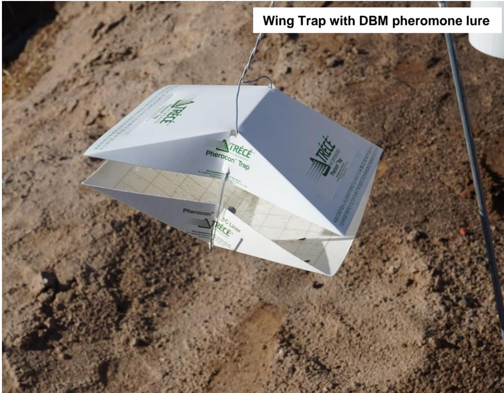
Wing Trap with DBM pheromone lure
