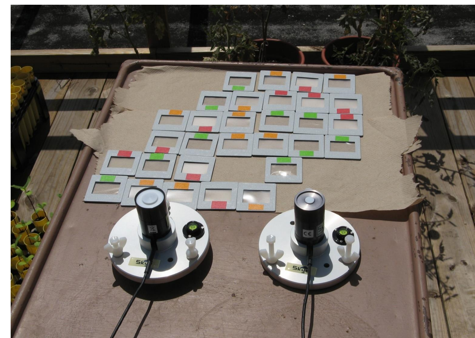
Fig. 1. Broadband sensors and polysulphone dosimeters in field test.
