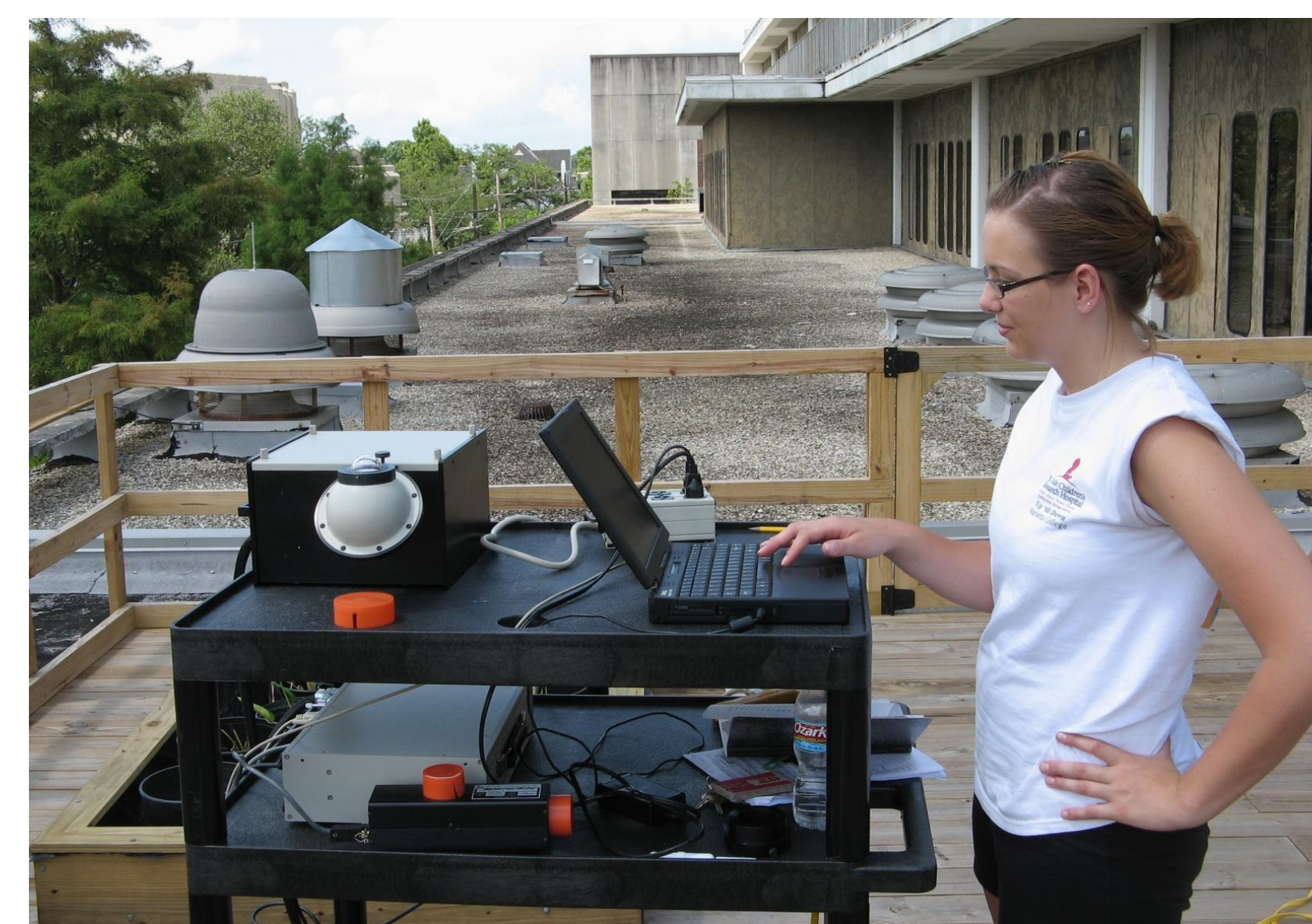
Fig. 2. Calibrating the broadband UV sensors using a spectroradiometer.
