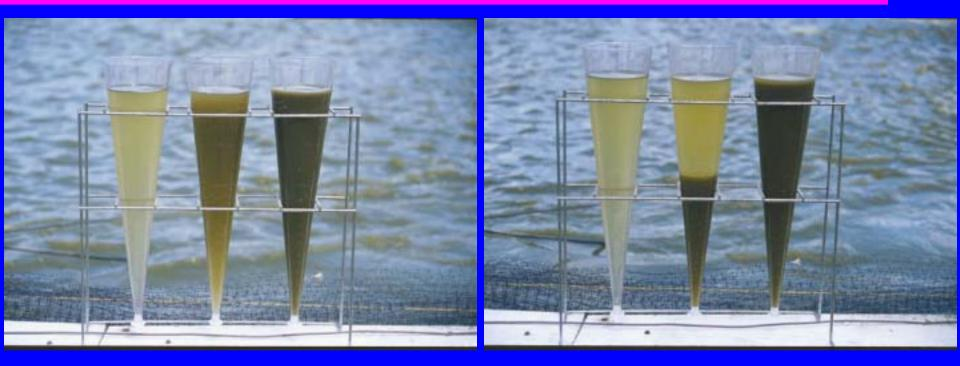
Clarifier effluent Culture tank water Sludge from clarifier
